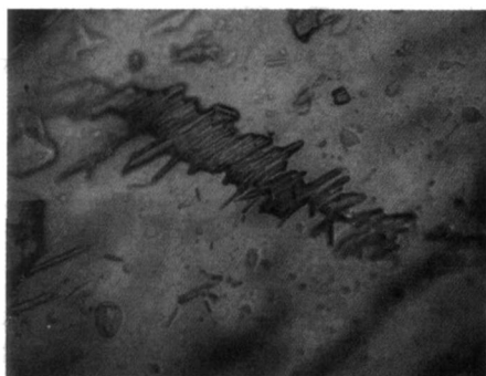
图 8 L-苹果酸脲晶体二维成核机制台阶生长的成核图 Fig. 8 Nucleation of ULMA crystal growing as two-dimension nucleation growth mechanism
