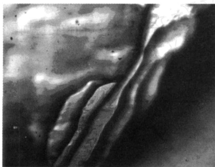
图 7 L-苹果酸脲晶体二维成核机制台阶生长 Fig. 7 Two-dimension nucleation growth mechanism of ULMA crystal
